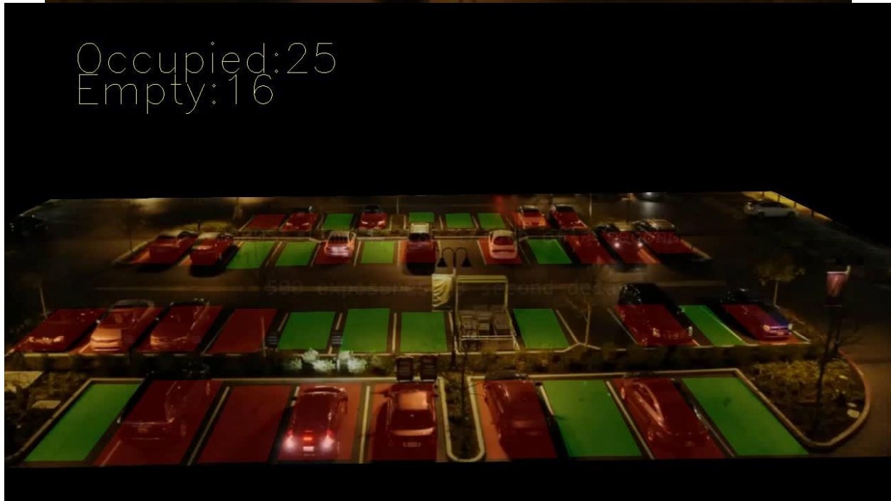
Figure 23. Night Parking Lot Masked without Perspective Transformation(top). Night Parking Lot Masked with Perspective Transformation (bottom).
