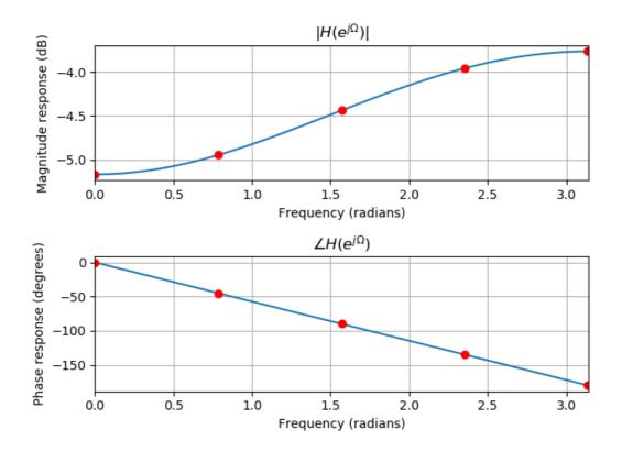
Design a five-tap FIR bandpass filter with a lower cutoff frequency of 1600 Hz, an upper cutoff
